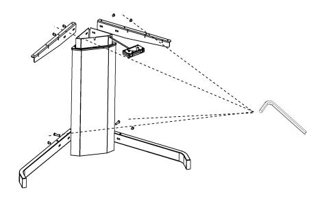
After the frame has been mounted the chosen tabletop is mounted and the operation unit will be possible to fix at the bottom side of the tabletop. This operation unit has to rocker switches.
